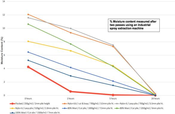
Diagram 2: Moisture content remaining after two passes using an industrial spray extraction machine
