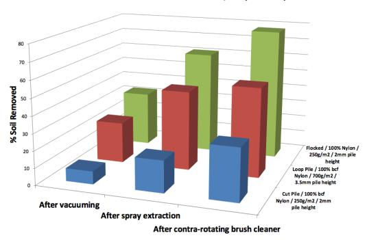
Diagram 1: Cleaning Research International - cleanability of flocked pile compared to other construction of Carpets
